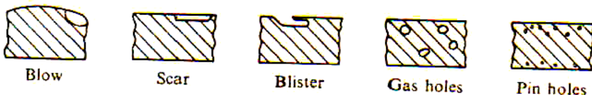
Fig. 10: Various gas defects
