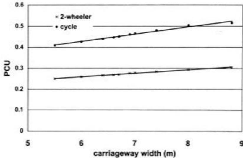
Fig. 2. Effect of carriageway width on PCU for cycle & 2-wheeler Classification of shoulders
