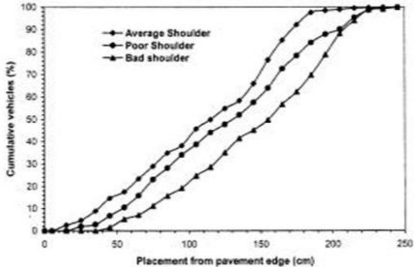
Fig. . Placement of car on two-lane road Reduction in speed during passing/overtaking manoeuvres
