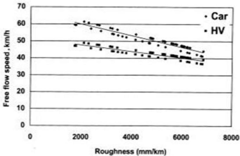
Fig. . Free flow speed related to road roughness
